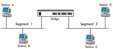
An Ethernet Bridge Connecting Two Segments
