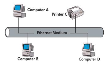
Since a signal on the Ethernet medium reaches every attached node, the destination address is critical to identify the intended recipient of the frame. For example, in the figure above, when computer B transmits to printer C, computers A and D will still receive and examine the frame. However, when a station first receives a frame, it checks the destination address to see if the frame is intended for itself. If it is not, the station discards the frame without even examining its contents.
